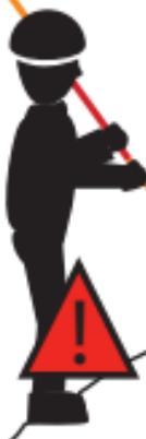
Probe perpendicular to the slope !
